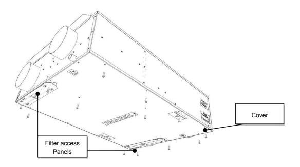
**Stage 1:** Isolate the mains power supply and remove the Filter access Panels and Filters.
