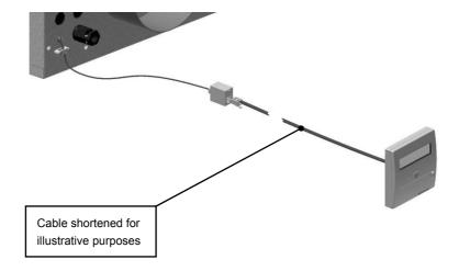
**3.** Connect the cable assembly to the Remote Control terminal block (the terminal block is colour coded to match the individual coloured cables and mount onto a single gang recessed wall box with the 2 screws provided.
